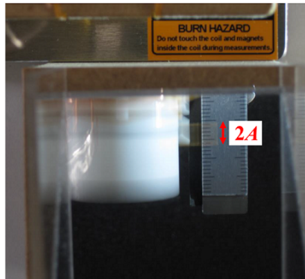
Figure 6: Oscillation behavior as seen through the mirror.
