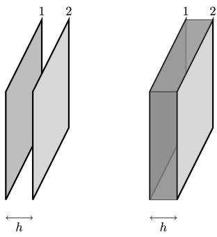
On the left is a simple model of two adjacent sheets 1 and 2 separated by a distance h. The sheets are not connected, and the perimeter is open to space. Assume the sheets are parallel. Thermal radiation can be exchanged between the sheets, and thermal radiation can escape through the perimeter gap. On the right, the perimeter gap has been shaded to help visualize.
