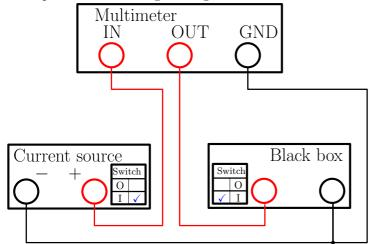
i. (1 pt) During charging of the capacitor from V = 0 to  $V = V_{\text{max}}$  we note that the output of the current source is constant ( $I_0 = 6.0 \text{ mA}$ ) close to the precision of the multimeter. ii. (1.2 pts) Using the definition of differential capacitance, we can calculate the current through the capacitor in the black box from the time derivative of the voltage on the black box.
