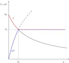
The rotation of the puck around its axis of symmetry is caused by the torque of the frictional force acting on the puck at the point of contact between the puck and the wall,  $M_f = rF_f = r\mu mv^2/R$ , where the radius of the puck r is the arm. The equation for the rotational motion of the puck, which results from Newton's second law  $Id\omega/dt = M_f$ , can be written as
