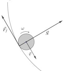
Let's focus on rolling with sliding first. The normal force  $\vec{N}$  of the wall on the puck is also perpendicular to the velocity of the puck at any instantaneous position of the puck. Force  $\vec{N}$  changes the direction of the velocity  $\vec{v}$ . From Newton's law in normal direction, we find  $N = mv^2/R$ , where m is the mass of the puck. Thus, the magnitude of the frictional force is  $F_f = \mu N = \mu mv^2/R$ .
