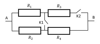
Subtracting (3) from (2),  $x(1+y)R - \frac{xRR}{xR+R} + xyR = 120 \ \Omega$ . After simplification,  $\frac{x^2R}{x+1} = 120 \ \Omega$ . Substituting *x* with the obtained value,  $R = 450 \ \Omega$ . Now substituting both *x* and *R* with their values in (2),  $\frac{2}{3}(1+y)450 \ \Omega = 400 \ \Omega$ , we
