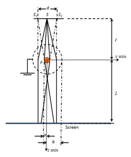
The electron "biprism" consists of a grounded cylindrical wire mesh with a fine filament *F* at the center. The distance between the source and the "biprism" is  $\ell$ , and the distance between the distance between is *L*.
