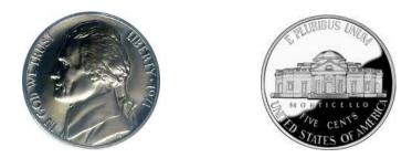
United States nickels (\$ 0.05 coins) consist of an alloy of nickel and copper (called "cupronickel"). Cupronickel alloys of similar composition are used for production of coins is some other countries. In this experiment you will determine the exact mass percentage of copper in a coin made of a copper-nickel alloy by dissolving the coin in nitric acid and determining the dissolved Cu(II) by iodometric titration.
