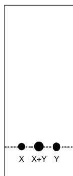
Fig. 1.1 Spots on the TLC plate before development; X: 1,4-DHP, Y: Reaction mixture.
