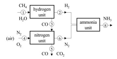
Assume that the reactants are converted completely. Take as flow for ammonia at position \$:  $n [NH_3, \$] = 1000 \text{ mol s}^{-1}$ .
