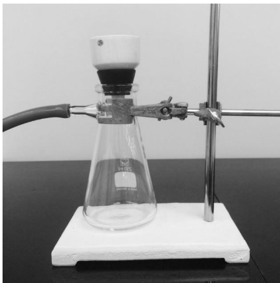
Figure 2: Set up needed for suction filtration.
